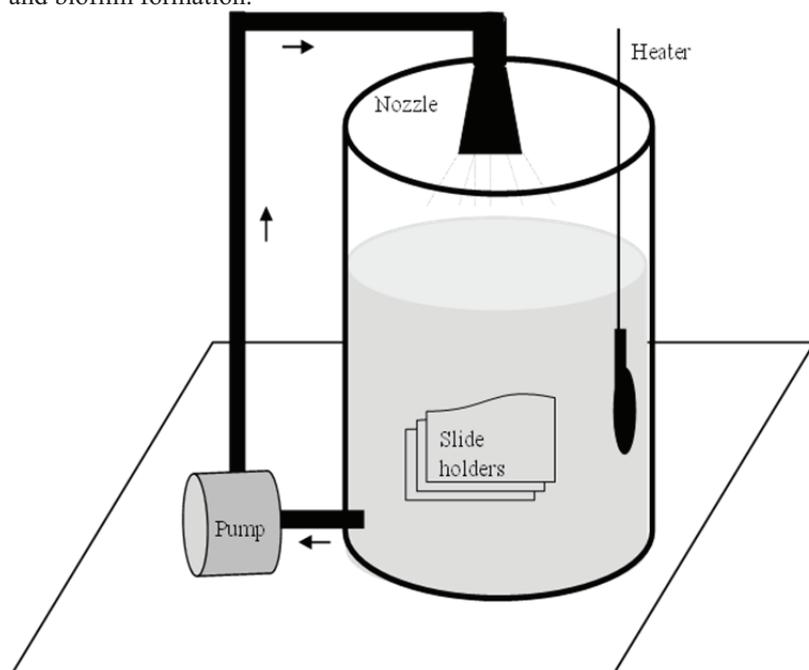
**Fig. 1** The schematic diagram of model recirculating water system, with arrows indicating the flow direction.
